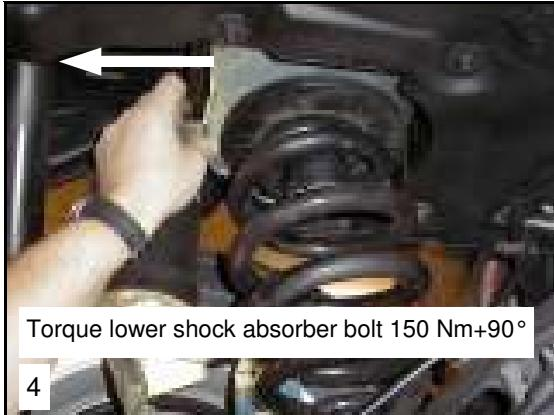
Torque lower shock absorber bolt 150 Nm+90°
